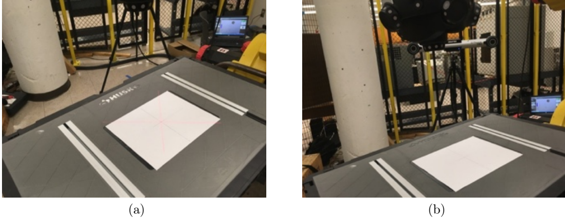
Figure 2.6: The robot calibrated and set up at zero position with the scanner installed and the table placed with the laser beam in the zero position
