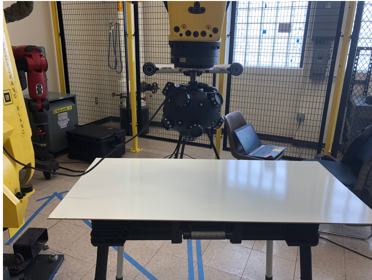
Figure 3.1: The Test Setup with the 3D scanner mounted to the robot and the white board as the flat surface
