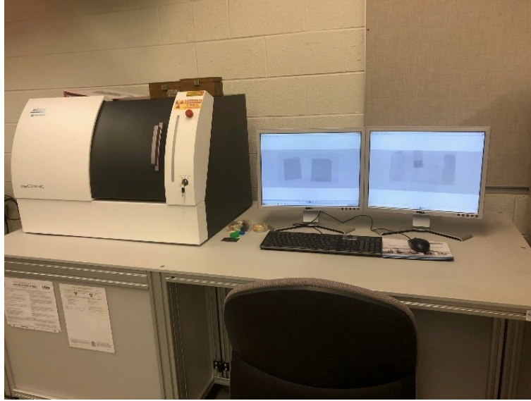
Figure 5.6: Wenzel exaCT-S device at Wayne State University
